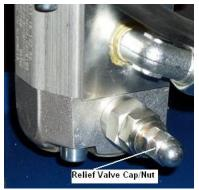
• Loosen the Locking Nut counter clock wise with a 13mm wrench.
