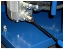
• Tighten Lock Nut in a clockwise rotation to fix the setting in place.
